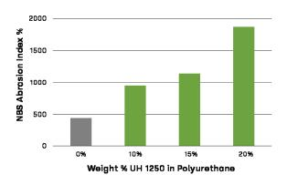
Addition of UH-1000 products to PU improves the wear resistance 4 times. Tested using NBS Abrasion Index (ASTM D1630).
