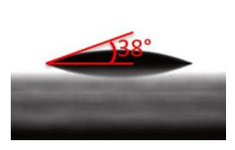
Increased surface energy of PP non-woven fabric treated by Inhance Technologies' ModySplash™ (on the top, surface energy is 28 dyne/cm (contact angle 98°), on the bottom, surface energy is 60 dyne/cm (contact angle 38°).
